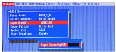
Note: Multiple arrays can be created using the same set of hard disk drives. The Capacity option allows you to set aside disk space that be used to create another array, set as a spare disk, or partitioned to act as a single disk (by the operating system).
